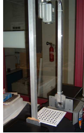
Figure 1: Turntable with calibration pattern
