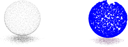
Figure 2: Two tangent surfaces: (Left) The original point cloud sampled from a sphere touching a plane. (Right) The two largest connected components extracted by the C2G pipeline: part of the sphere and part of the plane.
