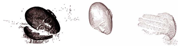
Figure 4: (Left) A cloud 3D point cloud obtained from stereo [3]; (Middle and Right) the two largest 2D components extracted from the 3D point cloud. The quality of the cloud segmentation into manifolds matches the one reported in [18].
